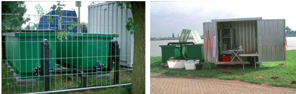
Figure 9 Migromat® at Linne with fence (left) and the Migromat® at Alphen (right): the container stores the reading devices and the computer equipment.
