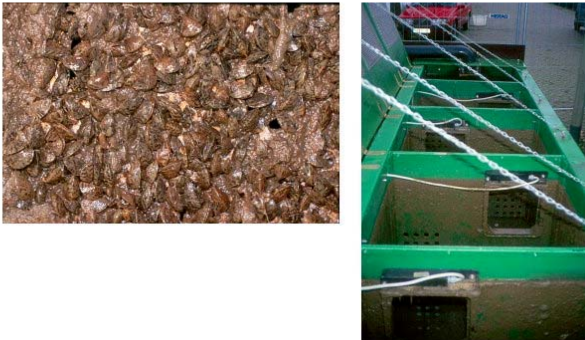
Figure 33 Dreissena polymorpha covering the outlet screens of the MM in Linne (left) and the deposition of mud inside of the tanks (right).
