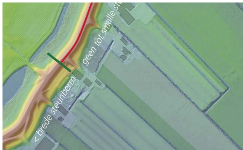
Overgangen dijkzone Achthoven west
