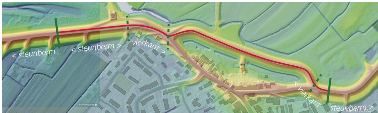
Overgangen dijkzone Lexmond
