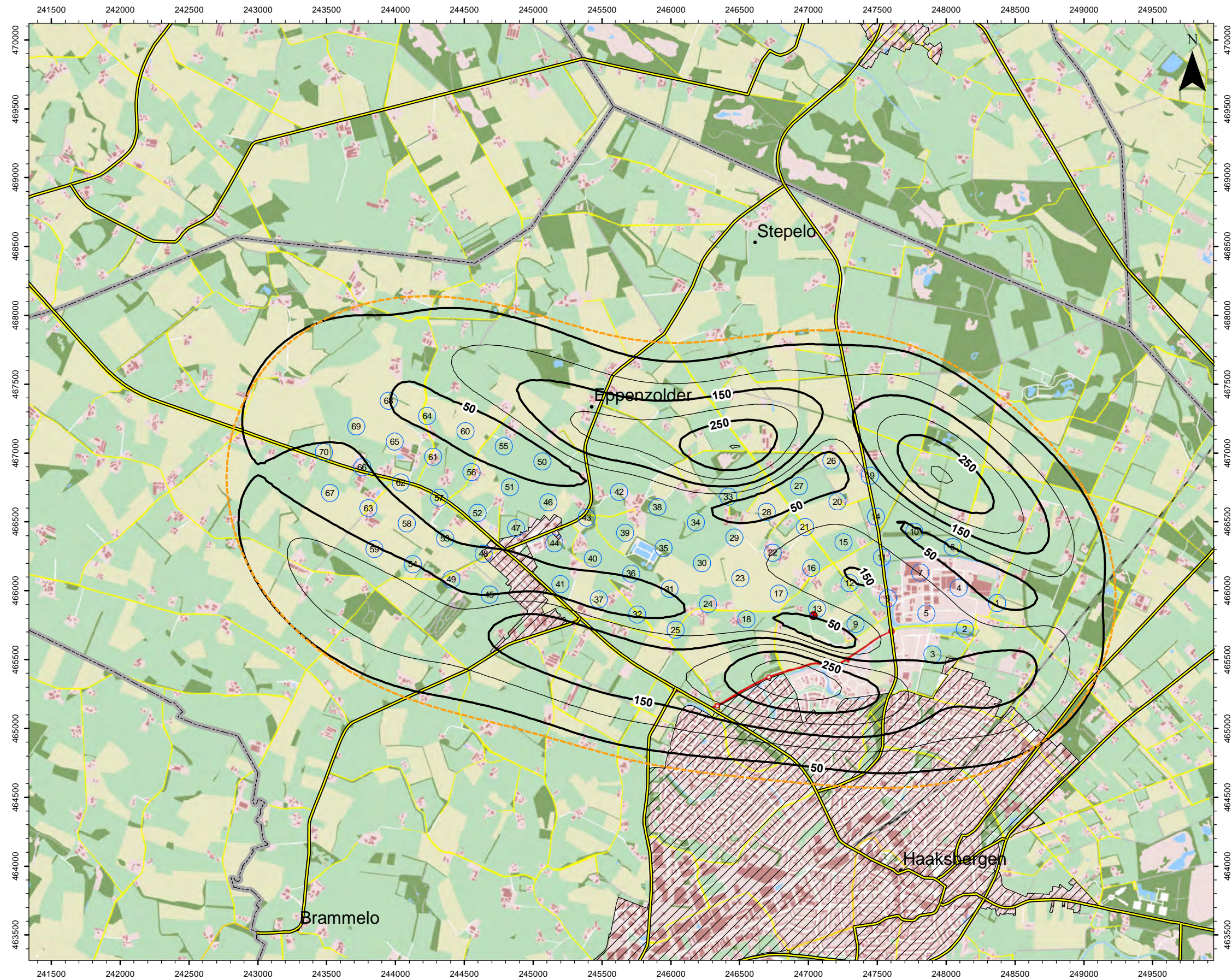
Enclosure 28: Isidorushoeve – Tensile strains [mm/km] – \beta=40^\circ – 100 years after start of production
