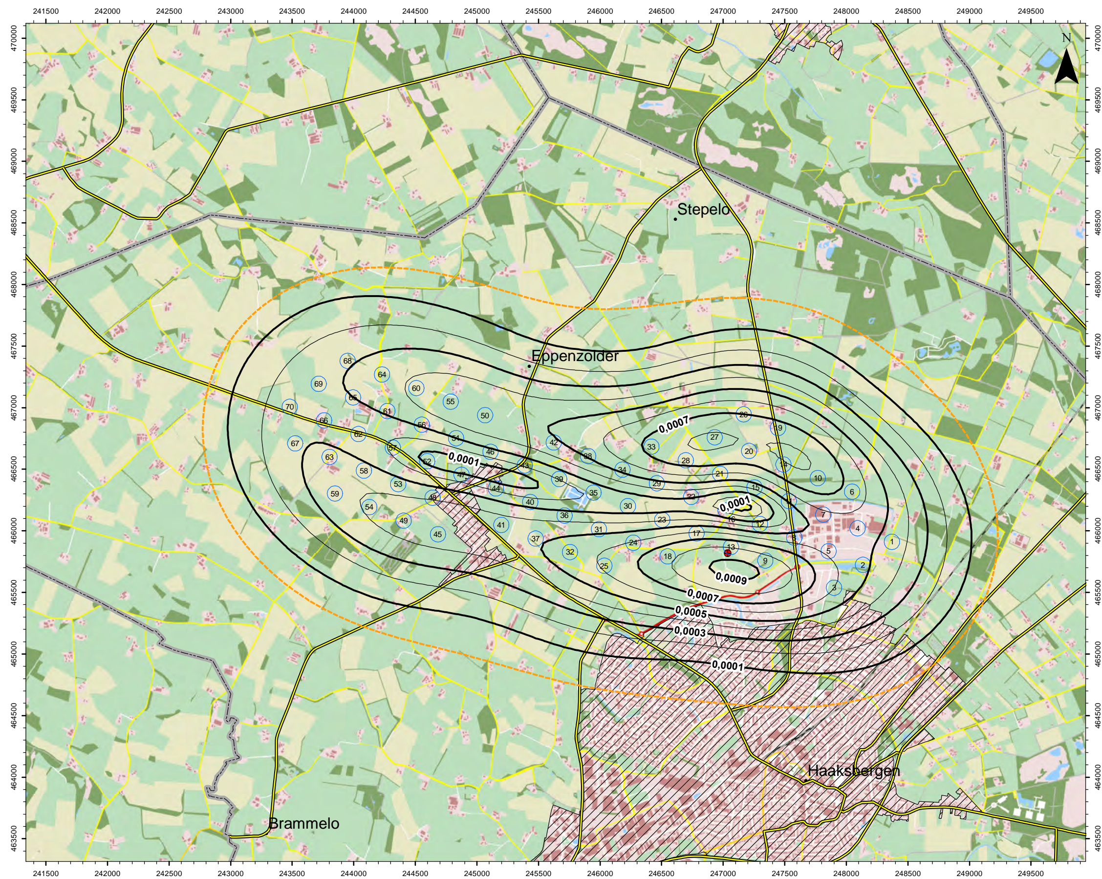
Enclosure 18: Isidorushoeve – Resulting tilts [m/m] – \beta=40^\circ – 100 years after start of production
