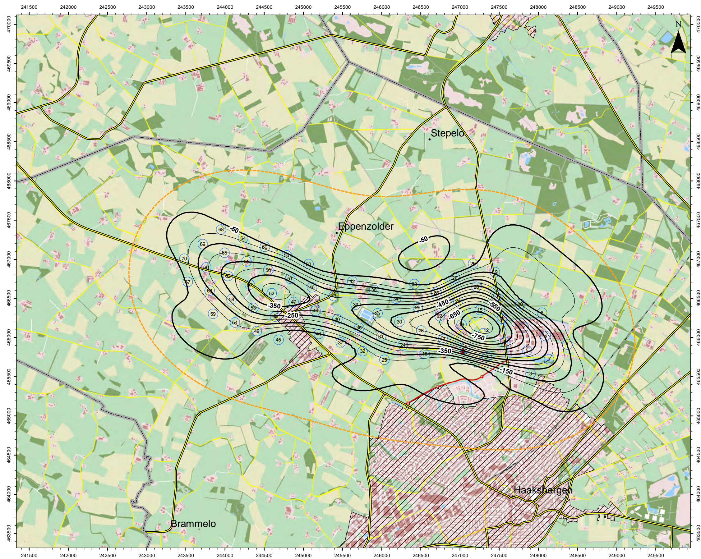
Enclosure 23: Isidorushoeve – Compressive strains [mm/km] – \beta=40^\circ – 100 years after start of production
