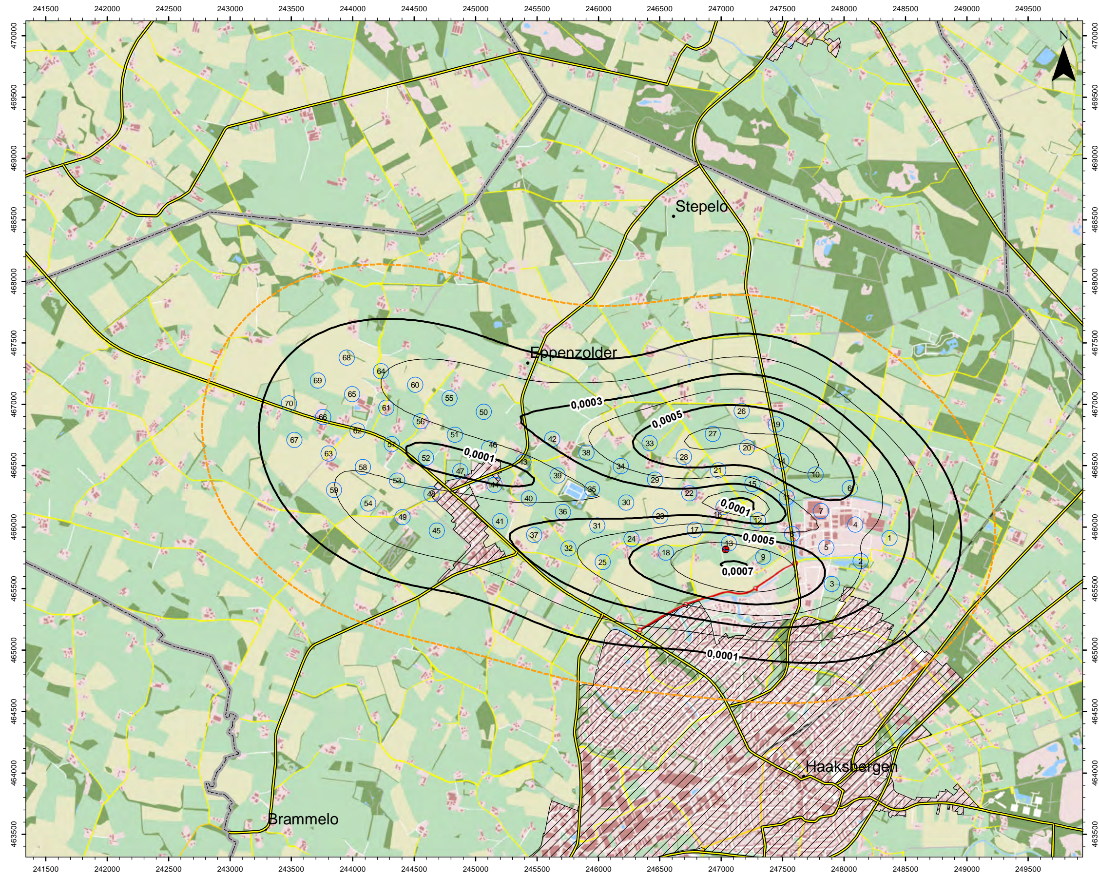
Enclosure 17: Isidorushoeve – Resulting tilts [m/m] – \beta=40^\circ – 75 years after start of production
