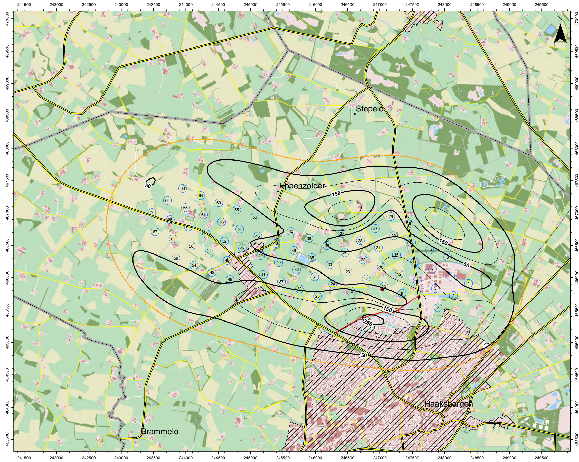
Enclosure 27: Isidorushoeve – Tensile strains [mm/km] – \beta=40^\circ – 75 years after start of production
