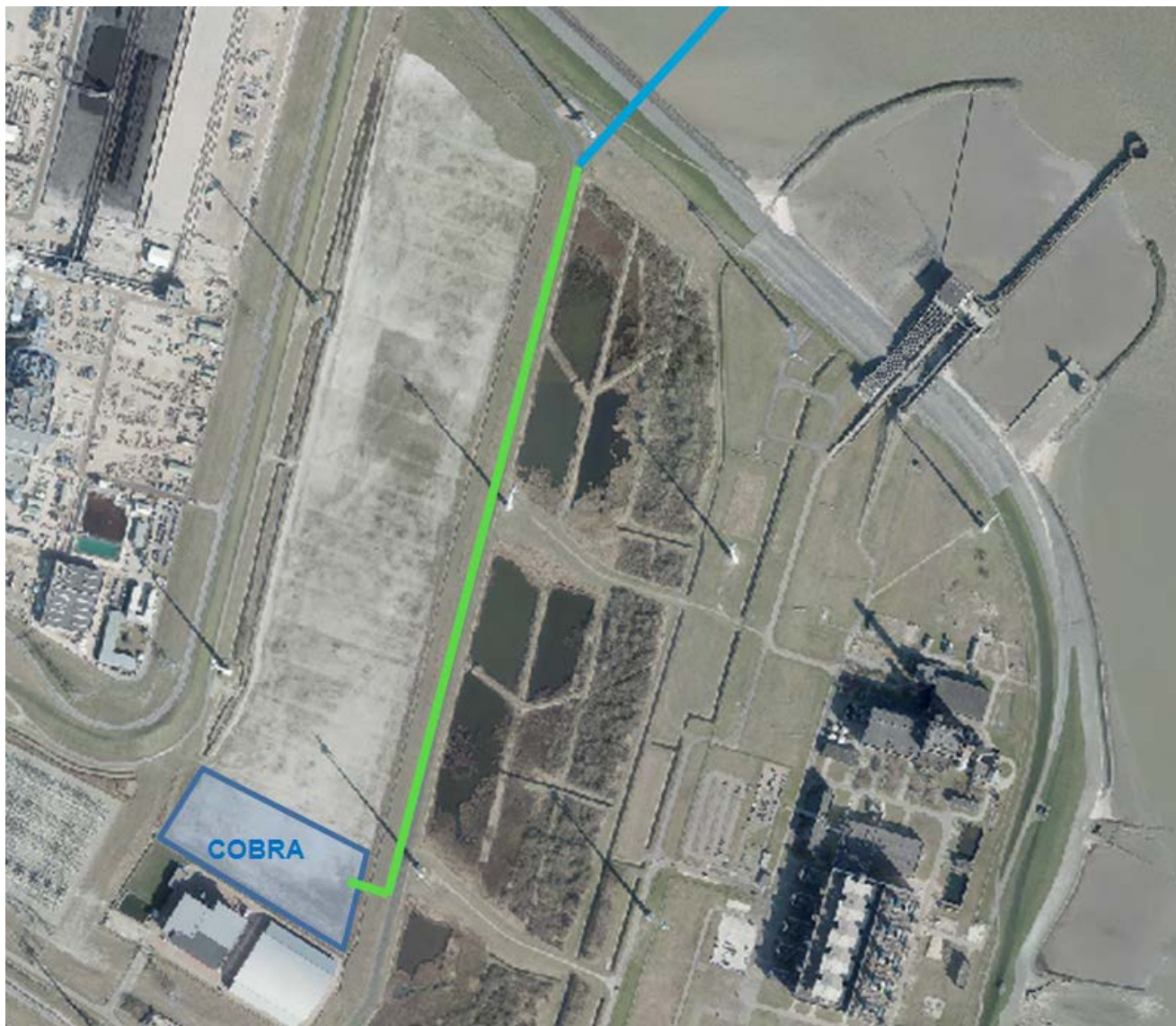
Figure 12 HVDC underground cable route (green)
