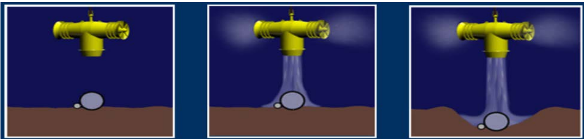
Figure 36 Mass flow excavation
