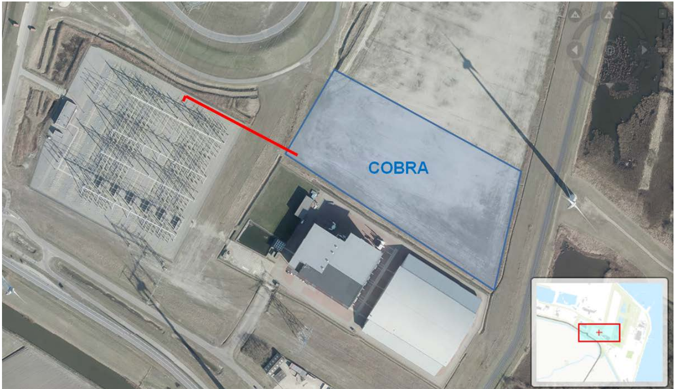
Figure 8 HVAC underground cable route (red)
