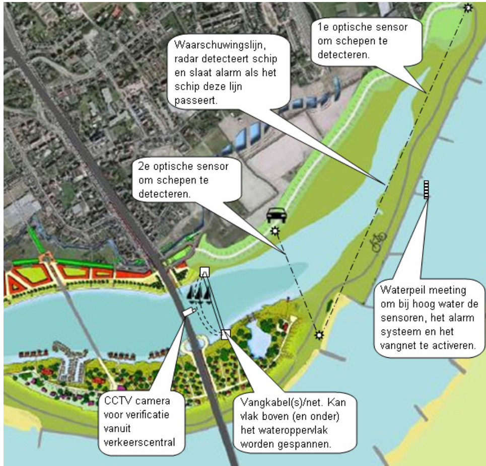
Figuur B2.9: Concept vangnet/vangkabels
